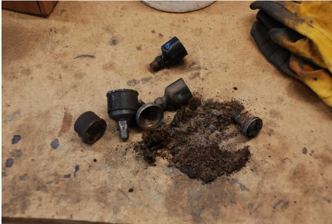
Gunk and Sand from Original Oil Cups
