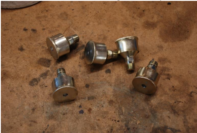
Replacement Oil cups modified and ready
