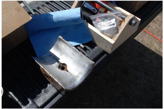
Journal Brass after removal and cleaning
