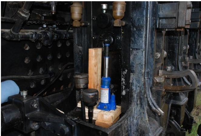
Jack Raising Crosshead and Connecting Rod
