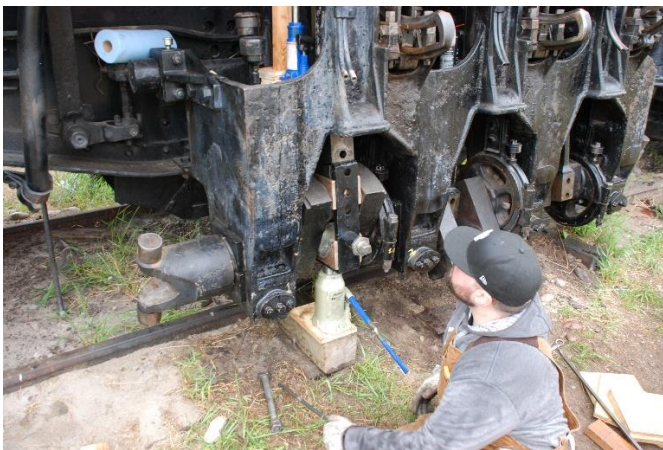
Jacking of # 1 strap into place
