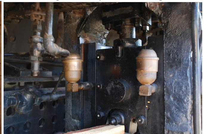
Larger Crosshead Oil Cups Cleaned and serviced
