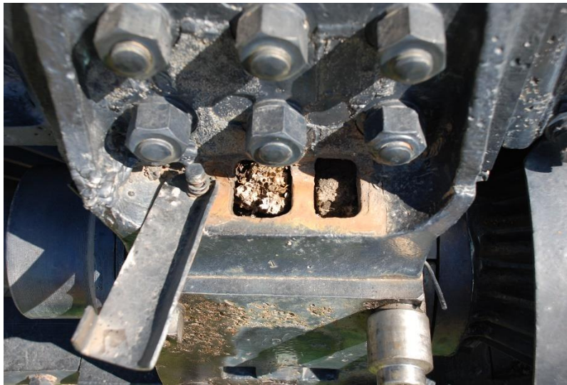
Debris in Journal Oil Gallery prior to cleaning
