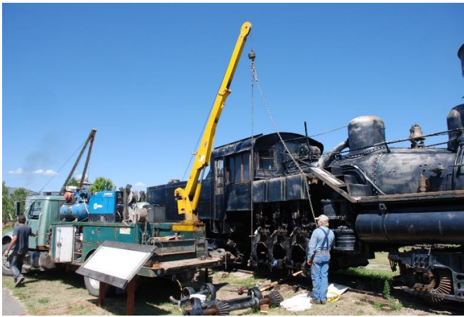
Rigging Crank to Crane for lifting
