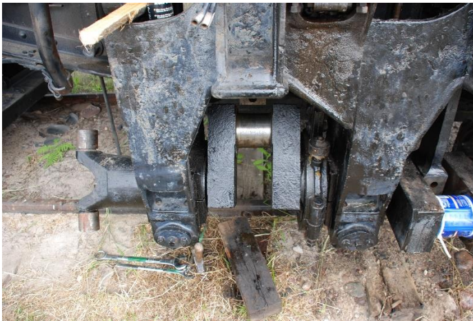
# 1 Crank Journal as found prior to cleaning
