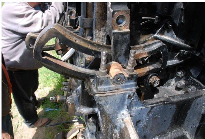
Link Block ready for cleaning cap removed
