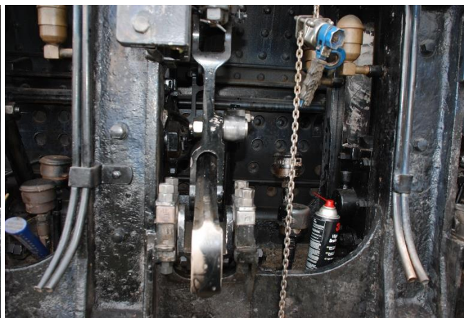
Link and blocks reinstalled after cleaning
